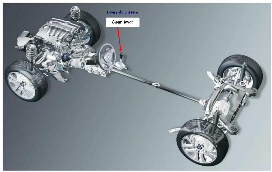
Situated in the passenger compartment, it allows the command of the gearbox..
