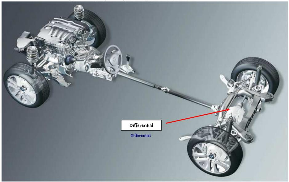
It dismissal the movement in 90 degrees and distributed the couple on driving wheels ...
