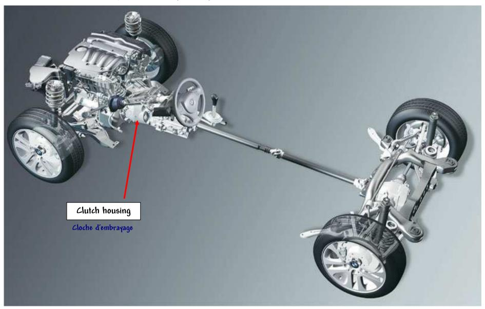
It is situated between the engine and the gearbox ... It is a crankcase ...
