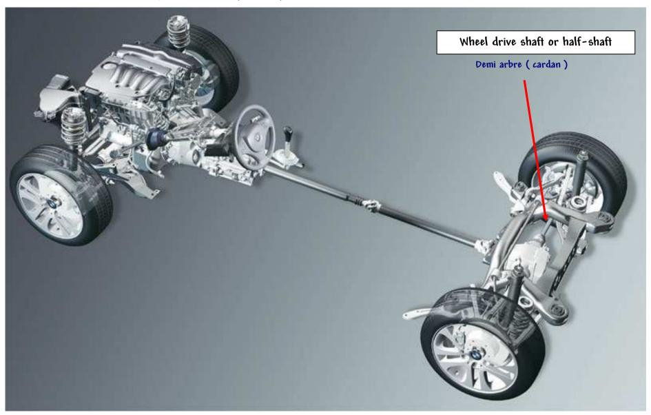
It passes on the speed and the engine torque up to driving wheels..
