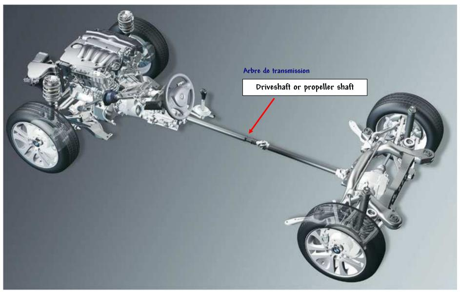
It passes on the rotation movement of the gearbox in the differential..
