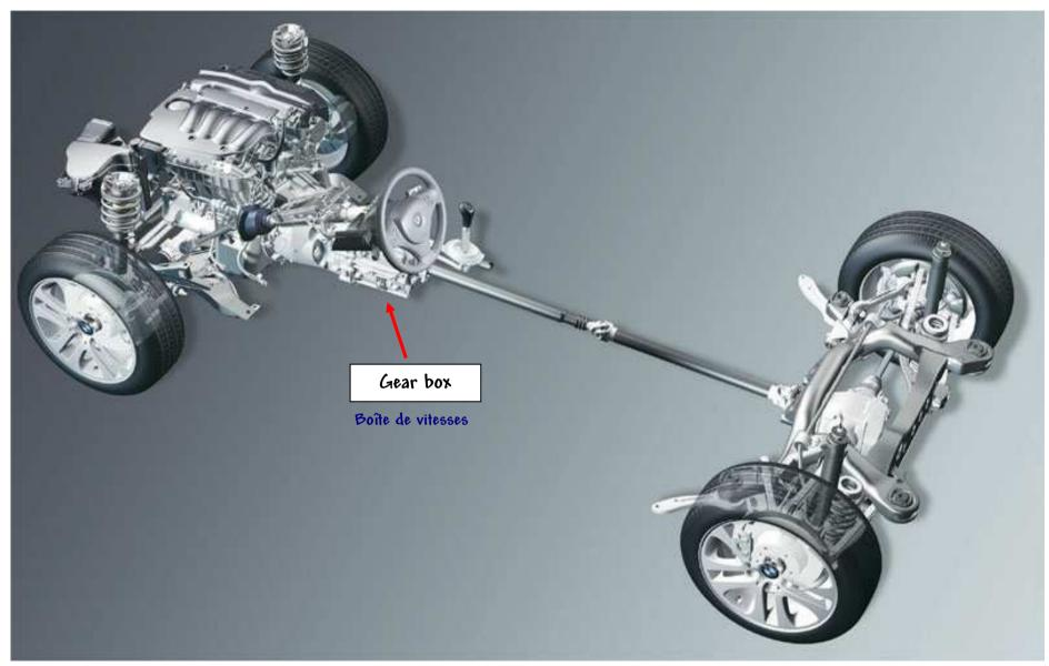
It adapts the engine torque to the resisting torque..
